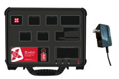
Open your Wi-Fi hub and ensure all the Camera's are in a slot. Remove the charger from the Wi-Fi hub.
