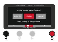
Standby mode: The system will turn off the Wi-Fi and other parts of the system. The Wi-Fi hub and camera's will remain charging.
