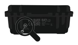
Unscrew the cap located on the back of the Wi-Fi hub. Connect the USB charging cable in to the slot. Connect the power supply to the mains supply.
